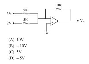
**29.** In the following circuit,  $V_i = 10mV$  dc maximum. The maximum possible dc output offset voltage is
